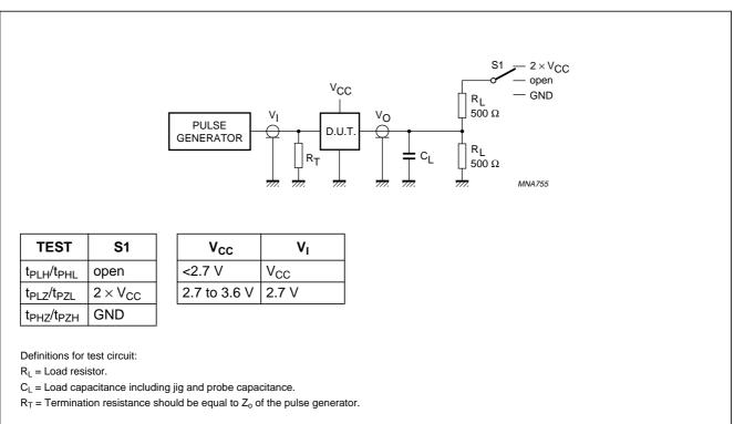
Fig.7 Load circuitry for switching times.
